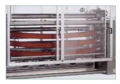
Products featuring exclusive CHIORINO technology, they provide the basic component of the expanding units with rotating bending rollers. They are particularly performing in the finishing machines, control phases of plastic films and apper processing mills:
